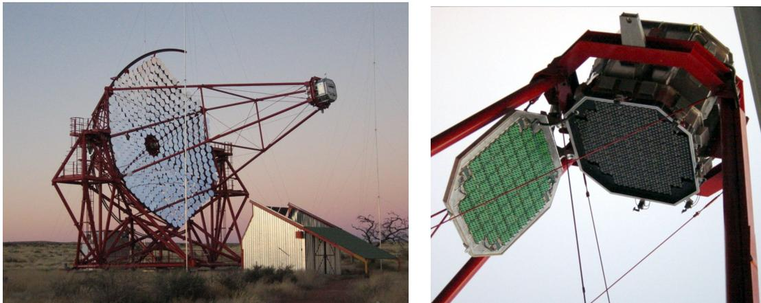
FIGURE 2.8: *Left Panel:* One of the telescopes of the H.E.S.S. experiment. During daytime the telescopes are positioned with the mast pointing towards the ground, so that the camera is parked in the small building on the right side of the image. *Right Panel:* Camera on the mast of a H.E.S.S. telescope. The open lid and the Winston cone plate (light guiding system) are visible. The PMTs are situated behind the Winston cone plate.
