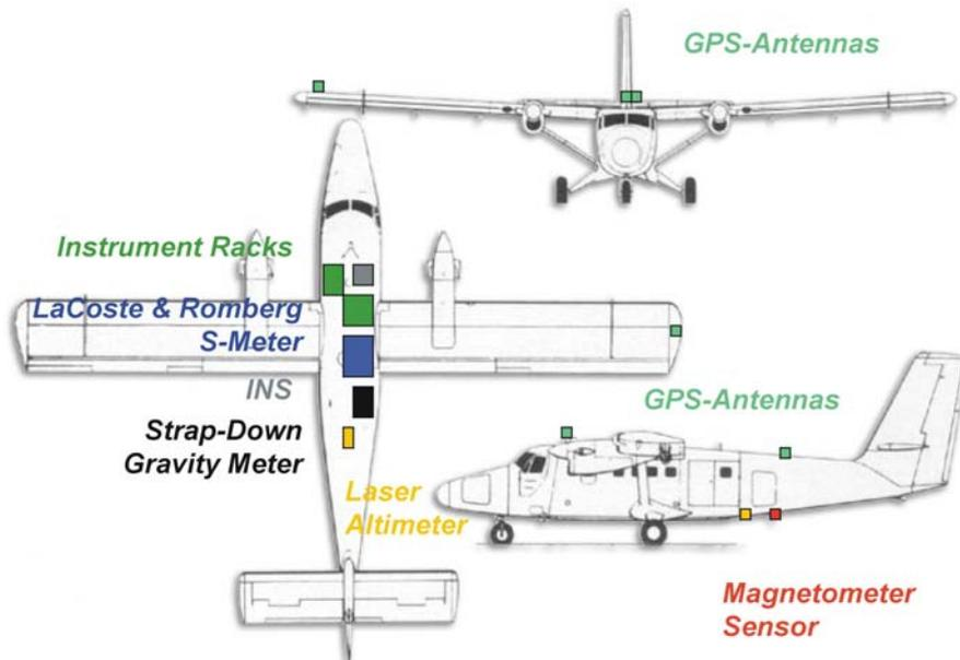
**Figure 4.2:** Mechanic installation of the ANGEL system in the SAF Twin Otter
