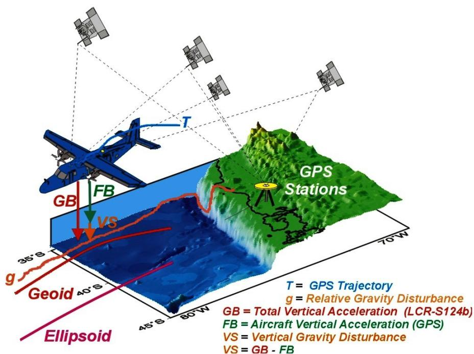
Figure 7.1: Overview about the concept of airborne gravimetry.
