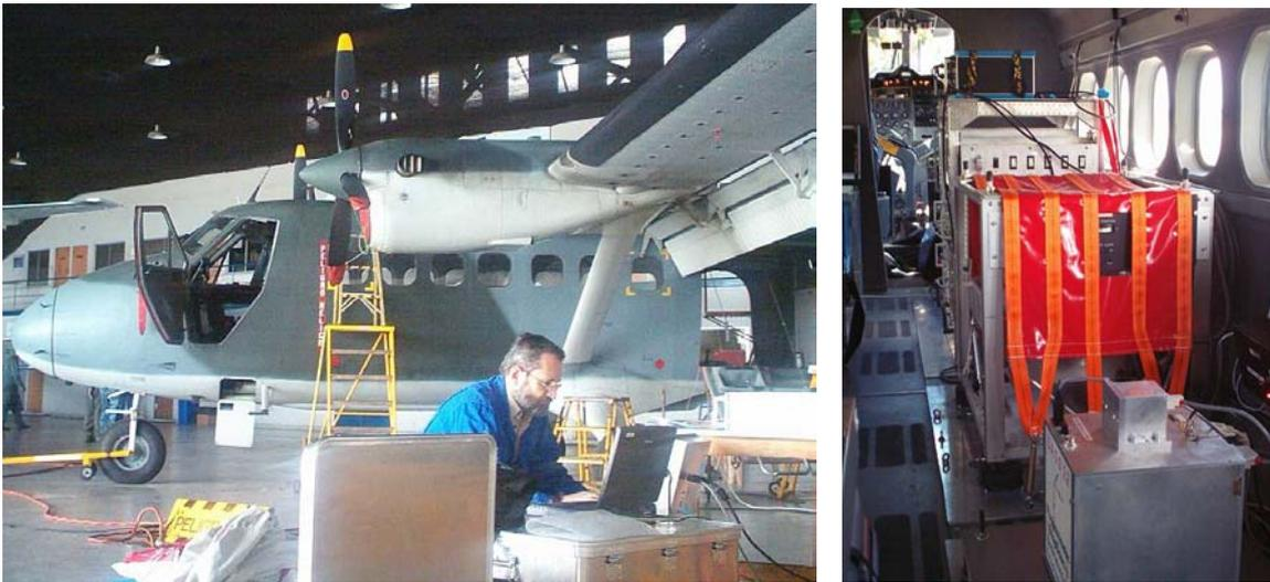
**Figure 4.1:** left: installation work; right: part of the installed equipment in the aircraft: at front SAGS 2.2 sensor, behind it LaCoste & Romberg gravity meter, in the rear the instrument rack.
