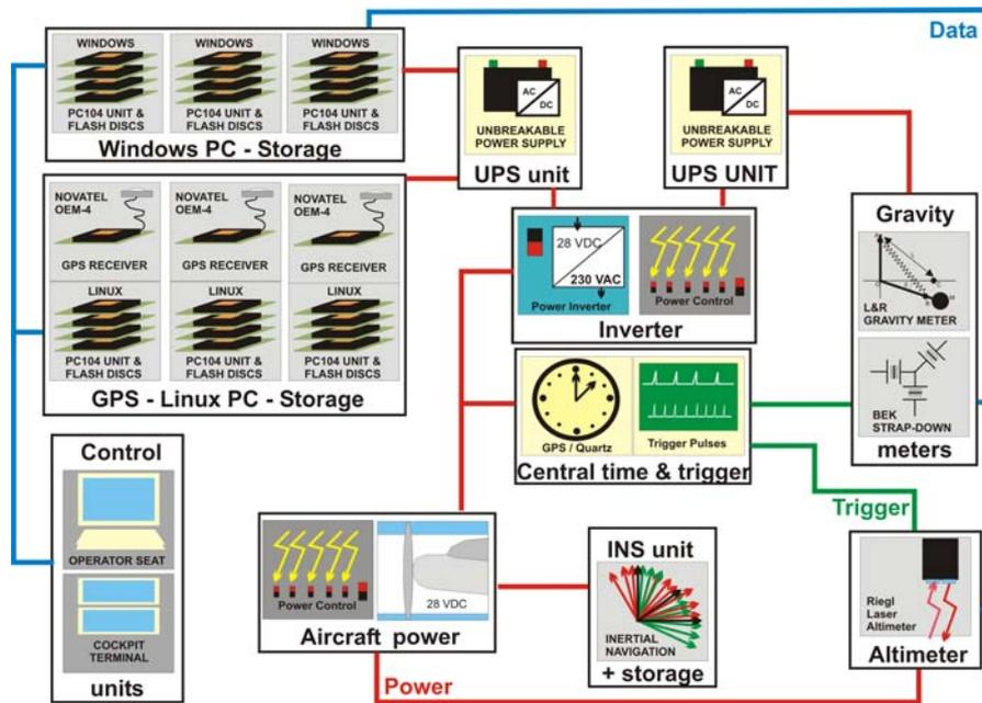
Figure 2.4: GFZ Potsdam airborne system components.
