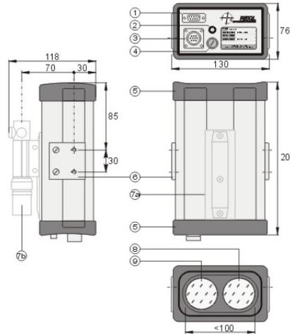
**Figure 5.10:** Riegl laser altimeter (physical units are mm).
