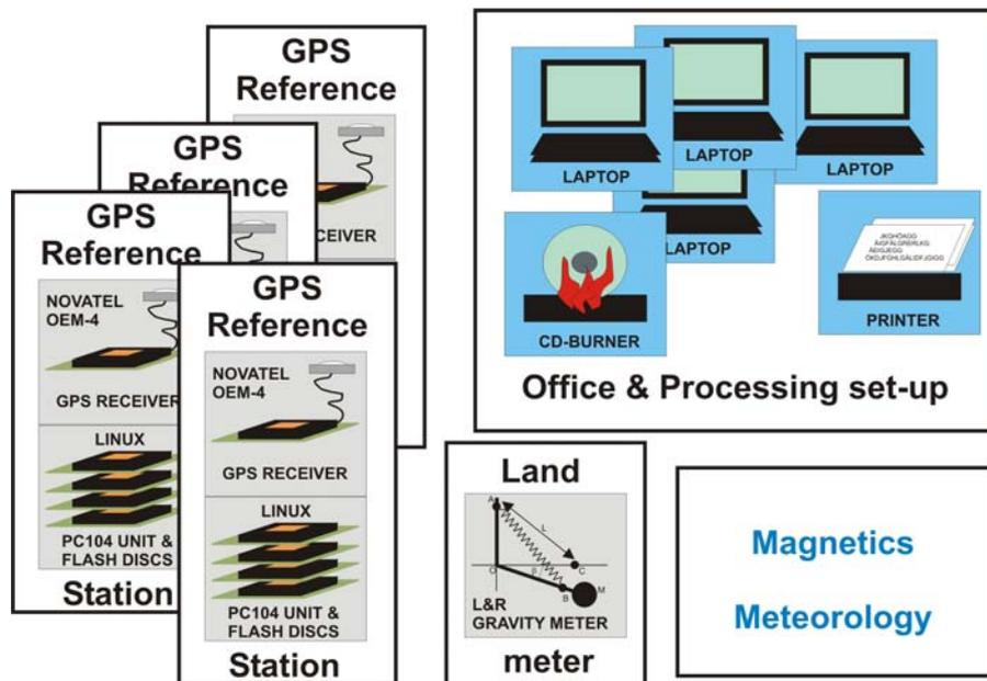
Figure 2.5: GFZ Potsdam ground system components.
