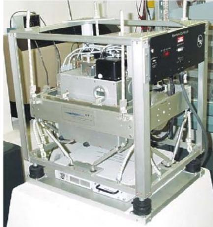
**Figure 5.2:** LaCoste & Romberg S124b gravity meter in GFZ laboratory
