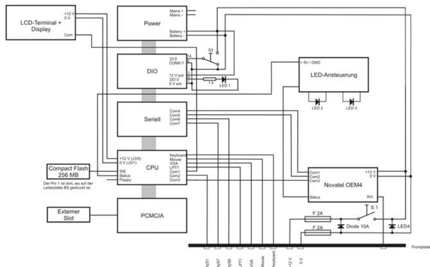
Figure 6.2: Internal architecture of the GFZ GPS ground reference stations.
