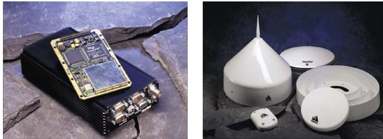
**Figure 5.8:** Novatel OEM4 GPS receiver and antennas. For the aircraft installation, the small flat antenna in left front is used, for the ground reference stations the in the right front in conjunction with the choke ring next to it.
