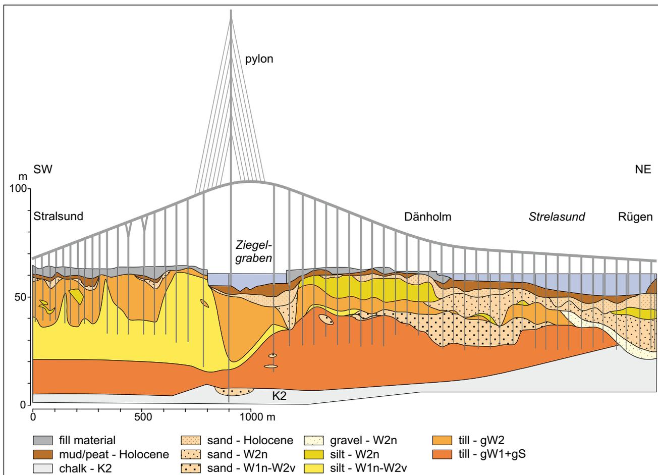
Fig. 3: Geological cross section (SW-NE) of the Strelasund (KRIENKE in NIEDERMEYER et al. 2010).
