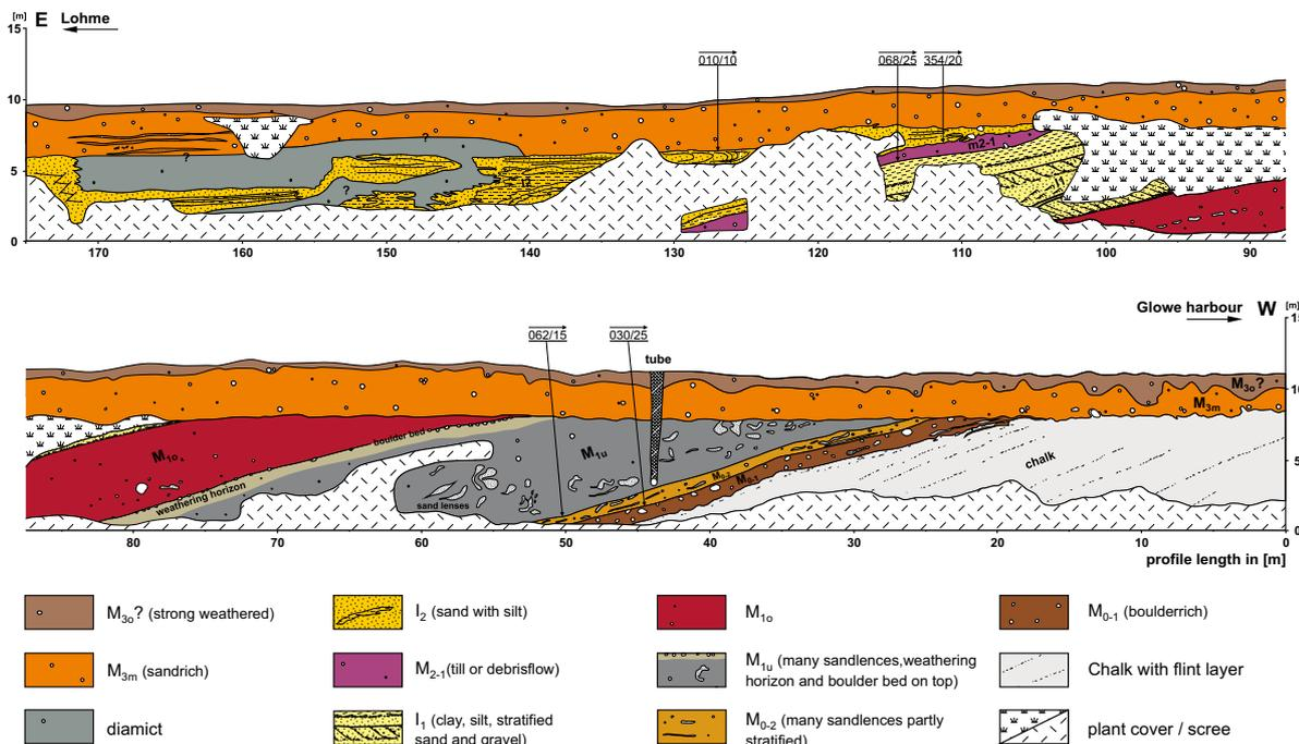
Fig. 4: Cliff section Glowe (re-mapped by KENZLER 2009/2010, NIEDERMEYER et al. 2010).
