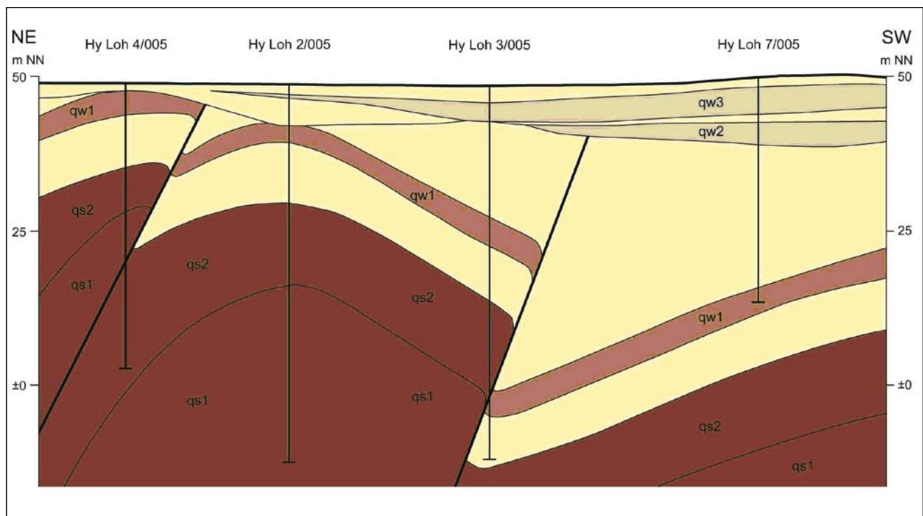
Fig. 7: Facies architecture of Saalian and Weichselian till units including chronostratigraphy (M, brown) as well intercalated glaciolimnic/-fluvial deposits (I-successions, yellow) at the Lohme cliff section (MÜLLER & OBST 2006, NIEDERMEYER et al. 2010).
