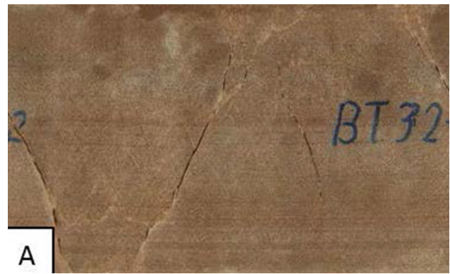
Fig. 4 Unrolled combined photographs of a sandstone sample after a multi-stage triaxial test [16]
