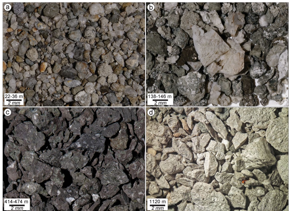
Fig. 14 Example of representative lithologies from the main geological units drilled at K-36: a from the 14 to 100-m depth, hyaloclastite consisting of mixed aphanitic basalt breccias and tuff; b from the 100 to 234-m depth, consolidated and greenish altered basaltic hyaloclastite (fine- and medium-grained tuffs), with abundant calcite; c from the 234 to 822-m depth, moderately altered, fine-medium grained basaltic lava with plagioclase phenocrysts; d white felsite fragments recovered at 1120 m drilling depth, with no clear evidence of intrusive contact with the host basalt. More data on the drilled lithologies discussed in the text are reported in Fig. ESM 4
