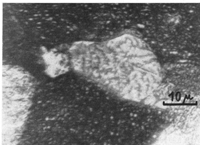
Fig. 7: Zigzag shaped domain boundaries on a crystal surface of a thermo-polished polycrystalline magnetite sample from Kirunavaara (Sweden).
