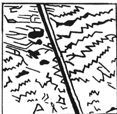
Fig. 4: Drawing of the zigzag shaped Bitter patterns of the area marked in Fig. 3.
