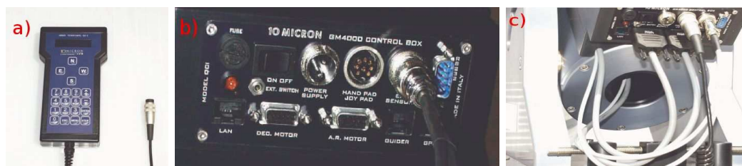
Figure 6.15: a) displays the handpad box which can be used to control the telescope at OCA, b) shows the ports of the mount, c) the channel inside the mount allows the secure routing of cables from instruments.
