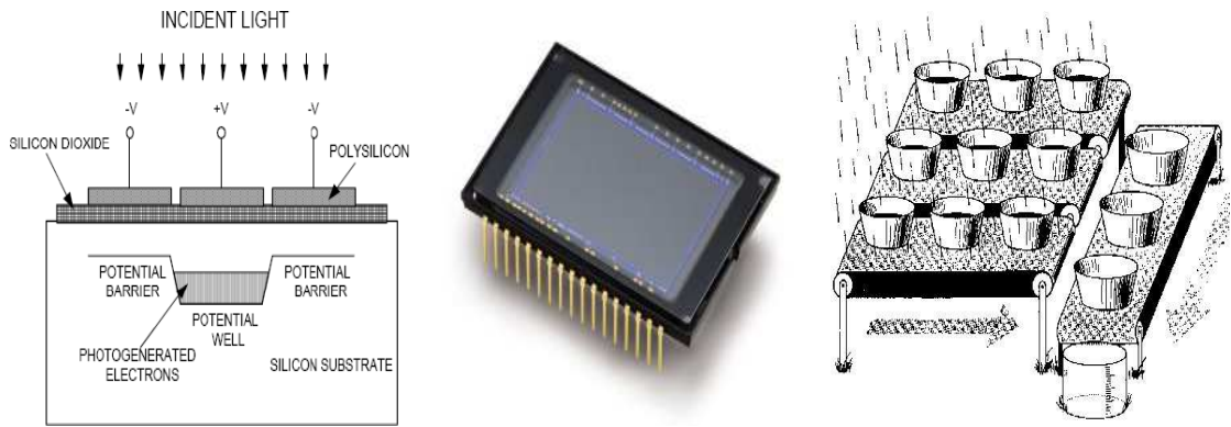
Figure 5.2: The function of a CCD chip is demonstrated in the left figure. The central figure shows a real CCD matrix consisting of single pixels. The principle of the readout of a CCD is shown in the right panel. Images taken from (163; 164).
