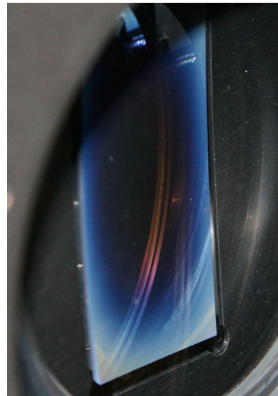
Figure 3.10: Contamination in the vacuum causing a bluish haze on the cold CCD surface before the cold head has been exchanged.
