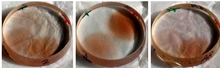
Figure 7.26: Samples number 2, 3, and 4 just after the tests. Darkening appeared in the spots radiated with high dose.
