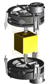
Figure 3.1: Caging mechanism. Source EADS Astrium.
