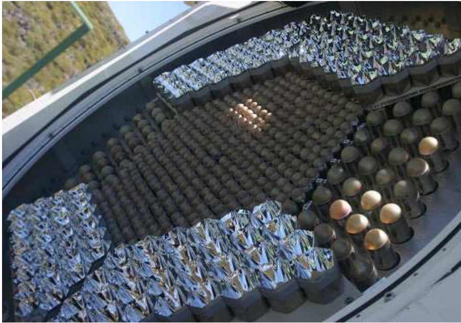
Figure 3.9: The camera of the MAGIC telescope in construction phase. The photomultipliers are partly equipped with Winston cones. Where sun-light is illuminating the PMTs the coating becomes visible.
