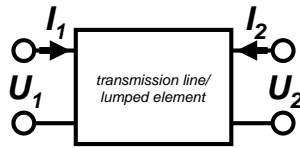
Fig. 3.13: Definition of currents I and voltages U at a 4-port using the ABCD-matrix convention.
