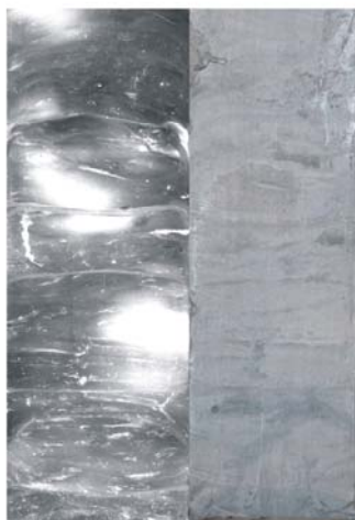
TB3 core, 38.2m: brown-grey coloured silt, thinly interlayer laminated sand/mud bedding, massive silt (TB2 core, 55m) organic material, mud clast (<1cm). bioturbation strong. Facies: intertidal flat
