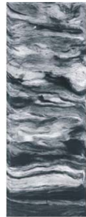
TB2 core, 60m: bluish red clayey silt with peat layers and lenses. Facies: mangro marsh (After Grothe, 2003)
