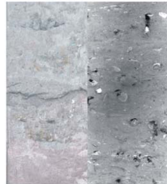
TB3 core, 16m depth: medium sand rich shell. Facies: sandy bar
