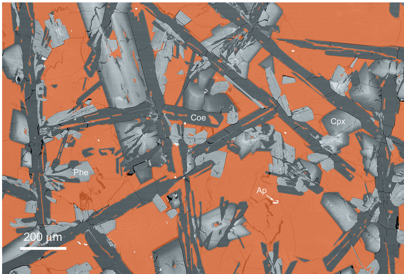
Figure 65: BSE image of Type 5 run G51 with a cooling rate of 0.3 °C/min and a bulk water content of 9.1 wt.%, run time 41.5 h, quenched at conditions of 3.5 GPa / 700 °C, no annealing. The fluid phase (orange) comprises 43 vol.%.
