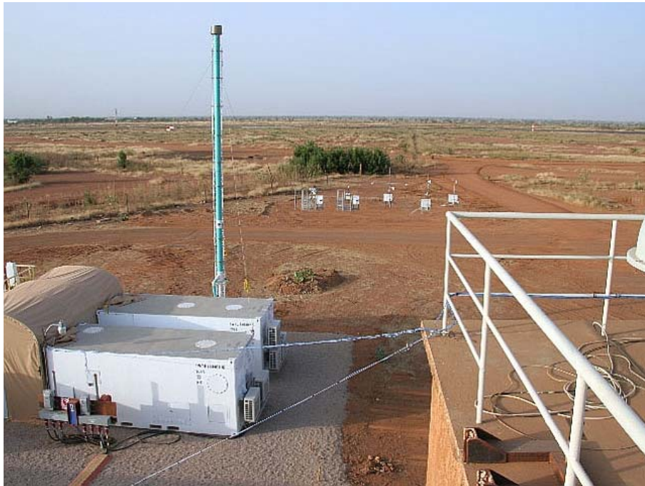
Figure 3.3: ARM mobile facility (AMF) in Niamey in November 2005 (shortly after deployment). In the front is the aerosol stack and the containers, in the background the AMF instrument field. Courtesy: U.S. Department of Energy's Atmospheric Radiation Measurement Program.
