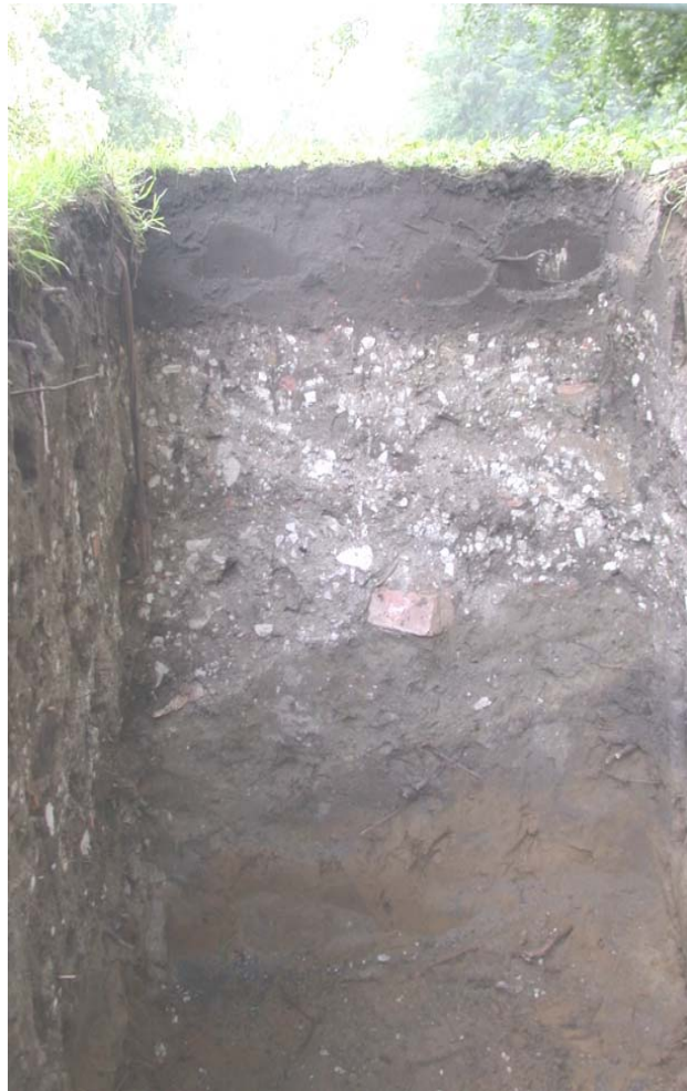
Figure 4.16: Exemplary soil profile of the INTERURBAN site Tiergarten, Berlin, Germany. Although the inclusions are not representative for the whole area, high soil heterogeneity is universally present.
