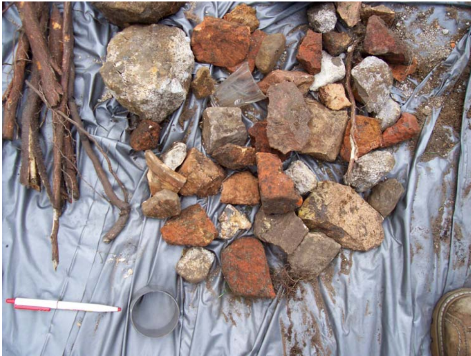
Figure 6.17: Assortment of various potential diffractors excavated at the INTERURBAN test site Tiergarten. The pen is pointing at a Kopecky cylinder with approximately 0.05 m diameter. Both the pen and the Kopecky cylinder are displayed for the purpose of comparison.
