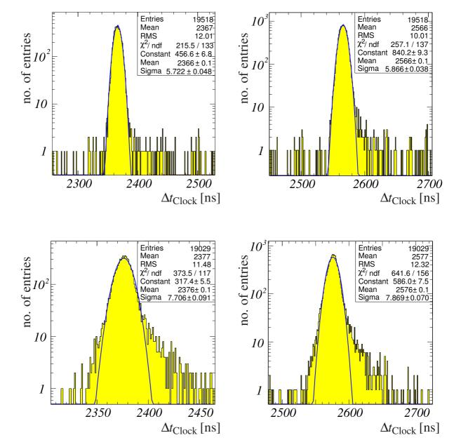
**Figure A.1:** Determination of the offset values by a Gaussian fit to the offset distributions. *Upper left:* Lower distribution of the offset between the  $e/\gamma$ -detector and Grande. *Upper right:* Upper offset distribution for the  $e/\gamma$ -detector. *Lower left:* Lower offset distribution for the  $\mu$ -detector. *Lower right:* Upper offset distribution for the  $\mu$ -detector.
