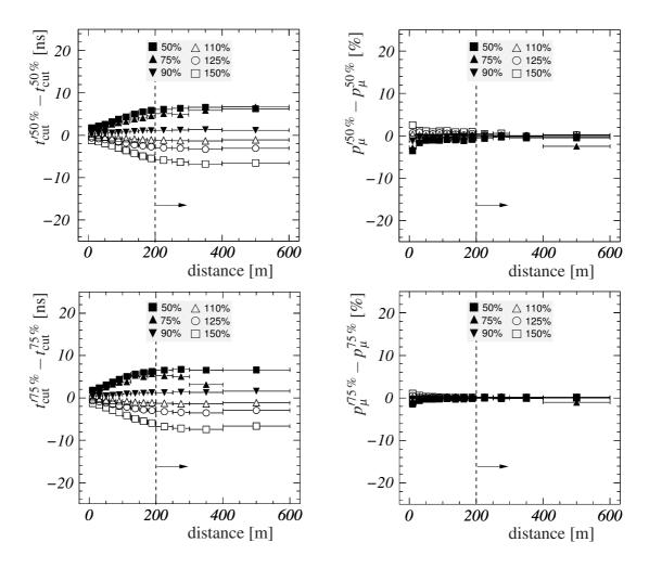
**Figure D.4:** Relative deviation of the separation cut values and the muon purities calculated from the 50 %-quantile and the 75 %-quantile for various sizes of the average MIP detector response. The dashed lines represent the core distance above which a separation of electrons and muons according to their arrival times becomes feasible.
