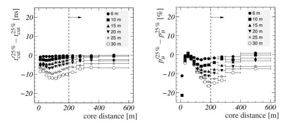
**Figure 9.13:** *Left:* Relative deviation of the separation cut values calculated from the 25 %quantile for various values of the core position smearing. *Right:* Relative deviation of the muon purities corresponding to the separation cut values for various values of the core position smearing. The dashed lines represent the core distance above which a separation of electrons and muons according to their arrival times becomes feasible.
