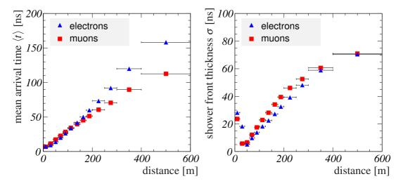
Figure 9.1: Left: Mean arrival time of electrons and muons as a function of the core distance according to the mean values of the particle arrival time distributions. Right: Thickness of the electromagnetic and muonic shower front as a function of the core distance in terms of the standard deviation of the particle arrival time distributions.
