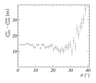
**Figure 8.6:** Difference between reconstructed and true shower core arrival time as function of the zenith angle. Due to the increase of the systematic deviation for  $\vartheta > 30^\circ$  only air showers with a smaller zenith angle are used for the analysis.
