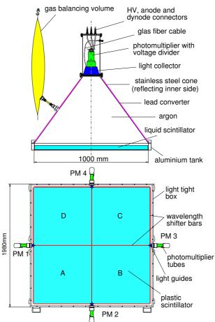
With the help of optical fibers brought into each cone the relative time delays between the detectors belonging to one cluster is determined by triggering all detectors simultaneously with laser pulses from a calibration system.
