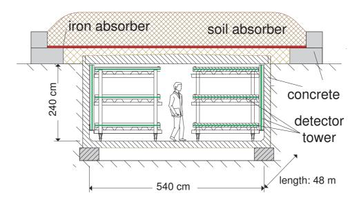
Figure 3.3: Schematic profile view of the muon tracking detector [Ant03b].
