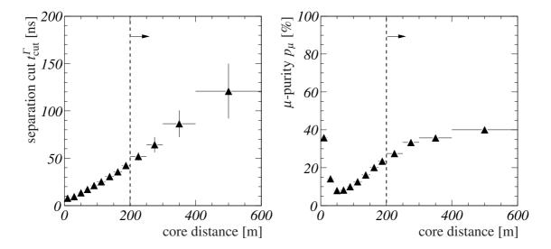
**Figure 9.6:** *Left:* Separation cut values as a function of the core distance. The cut represents the mean value of the mean values of the  $\Gamma$ -functions fitted to the electron and muon arrival time distributions. *Right:* Muon purities corresponding to the calculated separation cut values. The dashed lines represent the core distance above which a separation of electrons and muons according to their arrival times becomes feasible.
