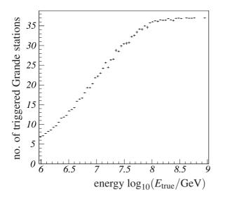
Figure **8.5:** Number of triggered Grande detector stations as a function of the simulated primary energy. From primary energies  $10^{16} \,\mathrm{eV}$  onwards, of air showers trigger on average at least 20 Grande detector stations.
