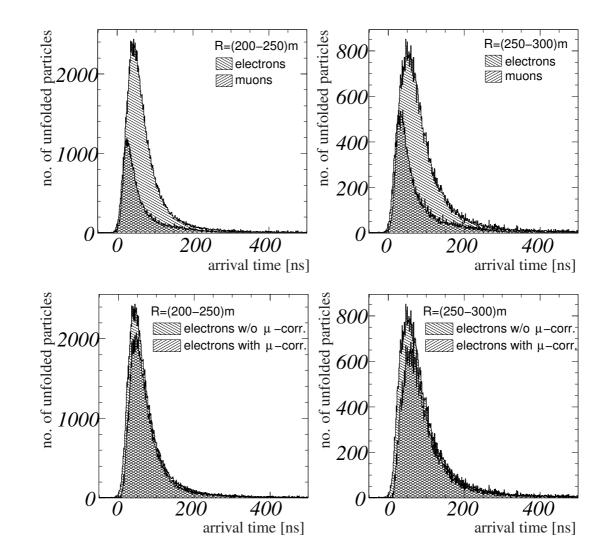
**Figure 8.8:** *Top:* Example arrival time distributions of the electromagnetic and muonic shower component, respectively, for two intervals of the distance to the shower core. *Bottom:* Illustration of the effect of the subtraction of the  $\mu$ -content from the distribution of the electromagnetic component. The distributions are shown for the same two intervals of distance from the shower core as in the upper part.
