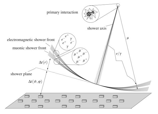
**Figure 2.6:** Scheme of the shower development in the atmosphere. Electrons have to cross a longer path length with respect to the point of the first interaction than muons to reach the same core distance. This leads to a time delay of the electrons. The difference in path length and thus also the time delay of electrons increases with the distance from the shower core.
