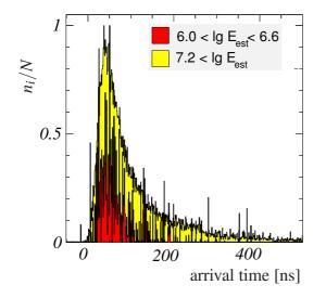
**Figure** 9.12: Muon arrival time distributions at core distances  $R > 300 \,\mathrm{m}$ for two ranges of the estimated primary energy. For better comparison, the bin contents  $n_i$  of distributions are the normalized by the total number of entries N.
