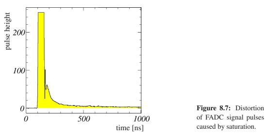
an upper cut on the signal amplitude at 240 pulse height units.
