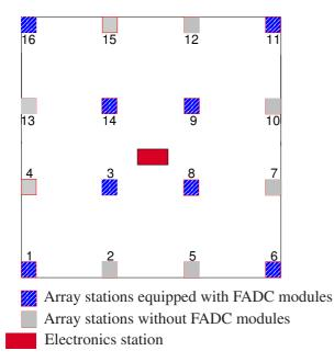
**Figure 4.1:** Distribution of KASCADE array stations equipped with FADC modules in cluster 1. The numbering scheme of the stations within the cluster is also shown.
