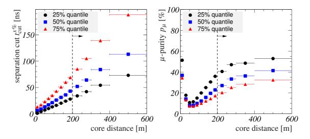
**Figure 9.3:** *Left:* Separation cut values  $t_{cut}^{x\%}$  calculated from the 25%-, 50%- and 75%quantiles of the electron and muon arrival time distributions. *Right:* Muon purities corresponding to the separation cut values calculated from the different quantiles. The dashed lines in both figures indicate the core distance above which a separation of muons and electrons according to their arrival time difference becomes feasible.
