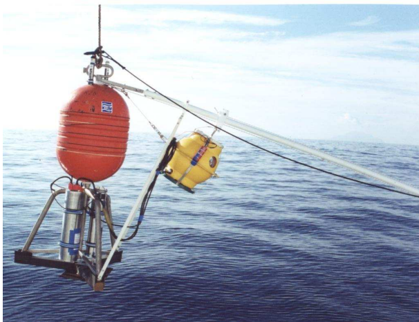
Figure 1.2: Ocean bottom station from GEOMAR, Kiel. A large floating body is located on top of a tripod. The seismometer is placed in an additional glass sphere as an external pack (yellow plastic sphere). Datalogger and Battery packs are placed in pressure tubes. Flash light and radio beacon are attached to top of the floating body.
