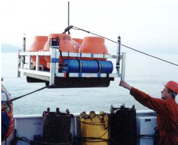
Figure 1.1: Ocean bottom station type Hamburg. Four glass floating spheres are located in the orange plastic shells. One of the glass spheres contains the seismometer. Datalogger and Battery packs are placed in pressure tubes (blue). Hydrophone, flash light, radio beacon and release transponder are attached to the edges of the frame.
