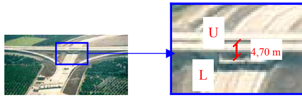
Figure 4-21: One of the Sample Constraints, Overpass-Height
