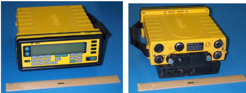
Figure 5.9: Trimble 4000 SSe Receiver Front and Rear View (Ruler Scale is 30cm)
