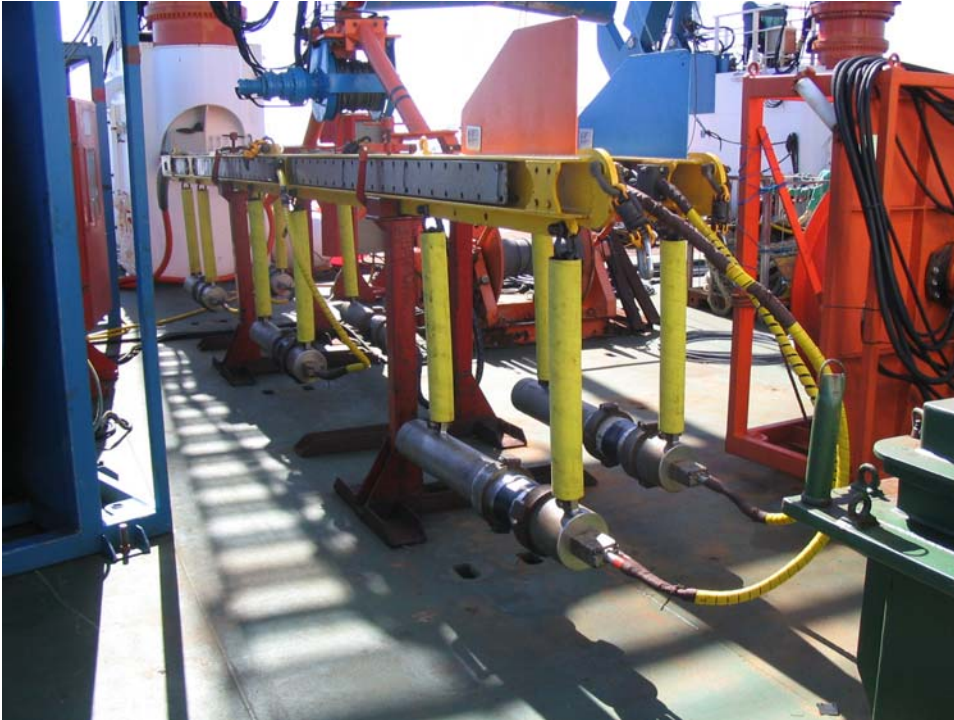
Figure 5.1.2.1: Picture of two airgun arrays with 3 guns each
