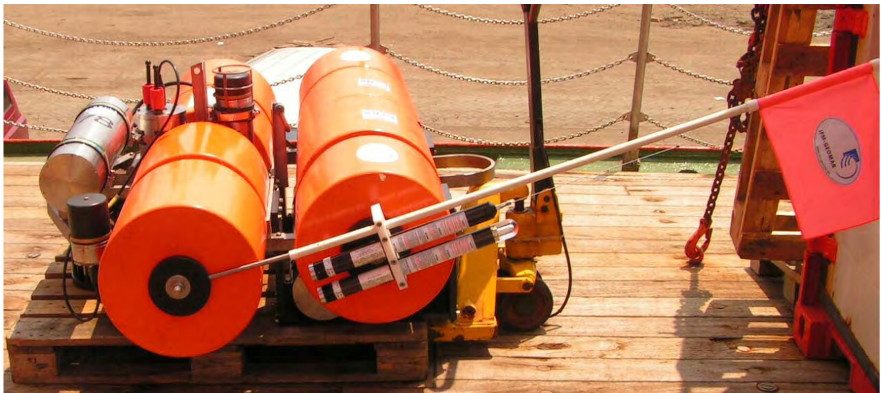
Figure 5.3.2: Instrument setup of the Ocean Bottom Unit. In addition to the Güralp Seismometer and a Differential Pressure Gauge, an acoustic device is mounted at the OBU to communicate with the surface buoy.
