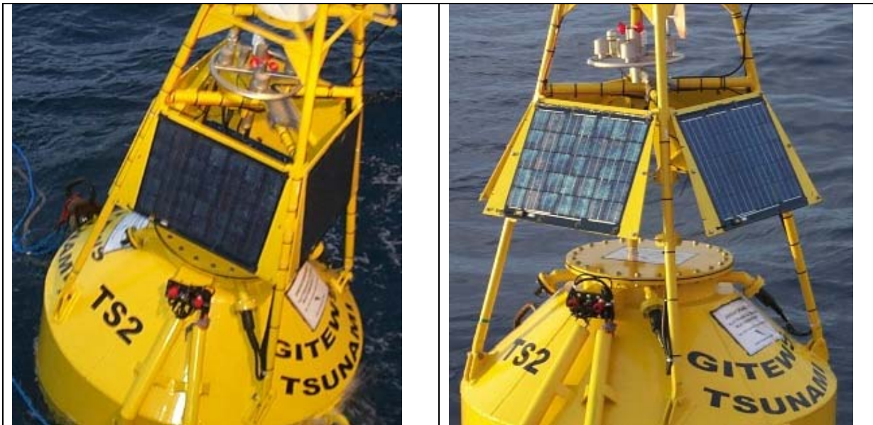
Fig. 6.7.3: Inclination of the solar arrays before and after the modifications; the lesser inclination will increase the recharging capability by about 10%.
