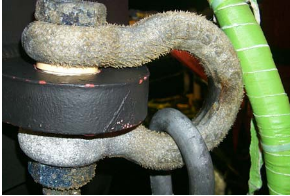
Buoy Connection Shackle, chafe in center
