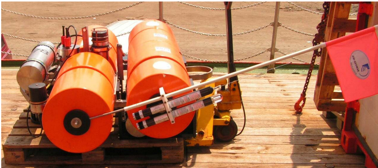
Fig. 6.5.3: Instrument setup of the Ocean Bottom Unit. In addition to the Güralp Seismometer and a Differential Pressure Gauge, an acoustic device is mounted at the OBU to communicate with the surface buoy.
