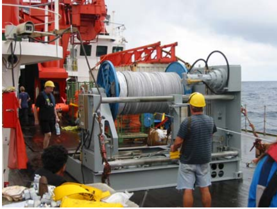
Spooling Winch deploying steel wire
