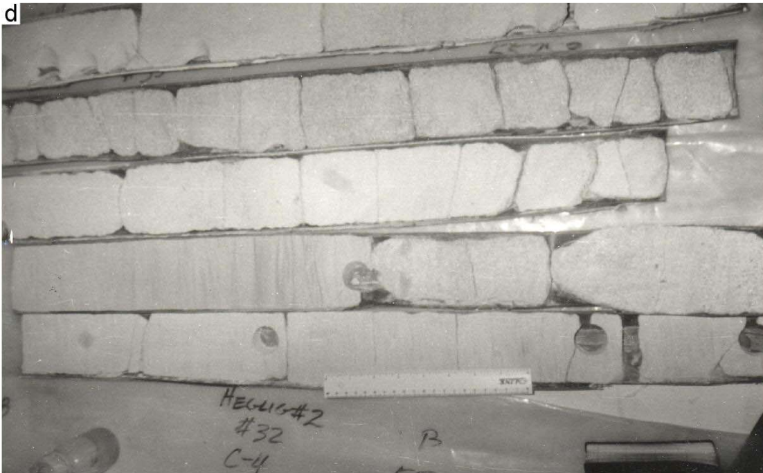
Photo. (d) Shows part of Core 4 from the Aradeiba Formation, Heglig-2 well in Heglig Field.
