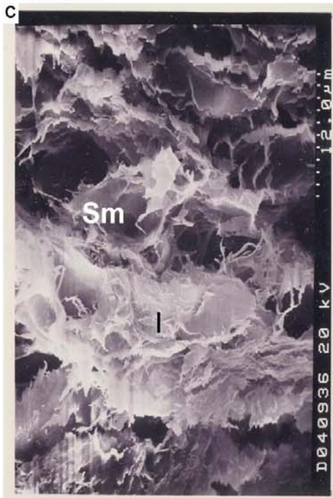
Micrograph (c) shows development of illite due to the transformation of the smectite to illite by burial diagenesis in a sample from the Aradeiba Formation at Talih-2 well in Unity Field.
