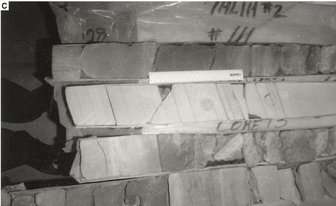
Photo. (c) Shows part of Core 13 from the Aradeiba Formation, Talih-2 well in Unity Field.
