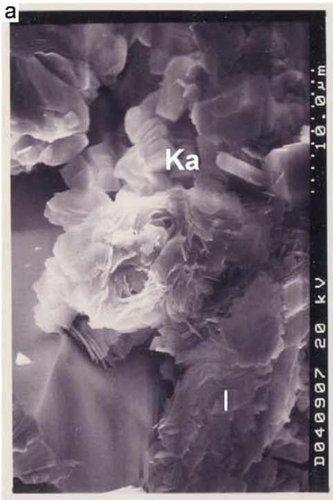
Micrograph (a) shows irregular flake-like clay platelets of illite forming a "scalloped" habit in a sample from the Zarga Formation at Talih-2 well in Unity Field.
