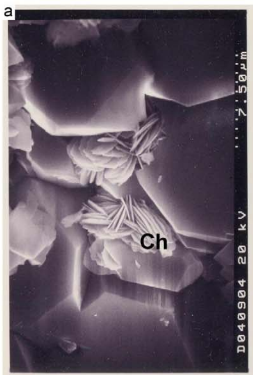
Micrograph (a) shows some clusters of "disc-like" chlorite crystals partly filling a depression within detrital grains in a sample from the Bentiu Formation at Heglig-2 well in Heglig Field.
