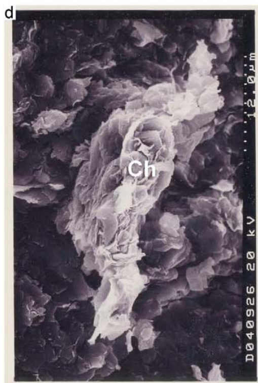
Micrograph (d) shows chloritization of biotite grain. the chlorite flakes were oriented face-to-face and aligned parallel to original biotite cleavage planes in a sample from the Aradeiba Formation at Heglig-2 well in Heglig Field.
