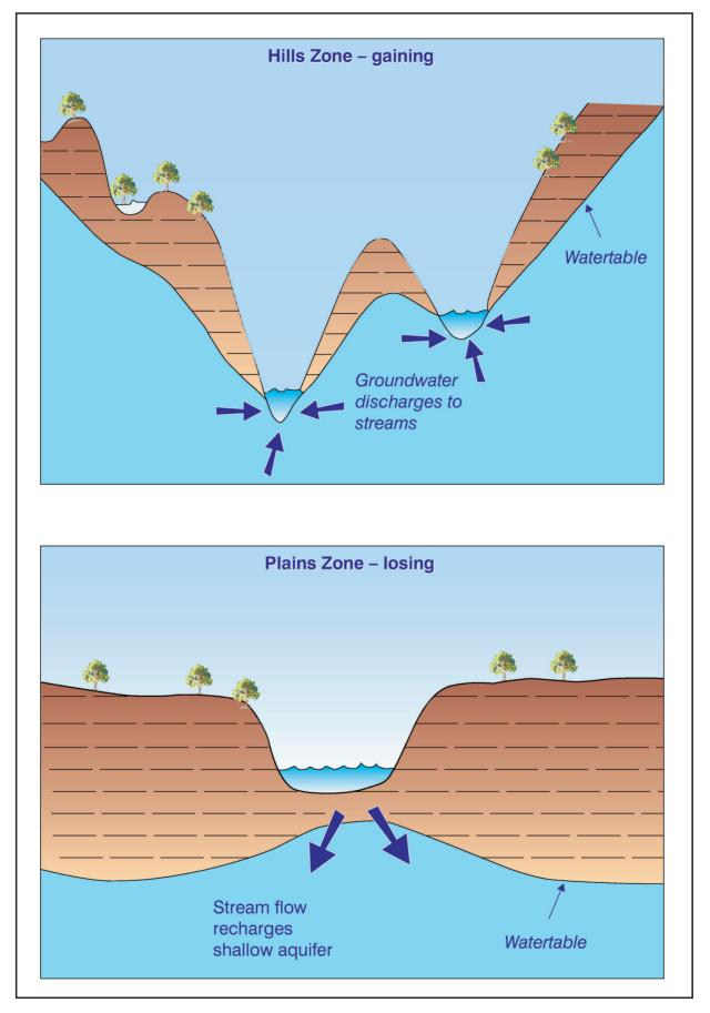
Figure 2. Groundwater - surface water interaction
