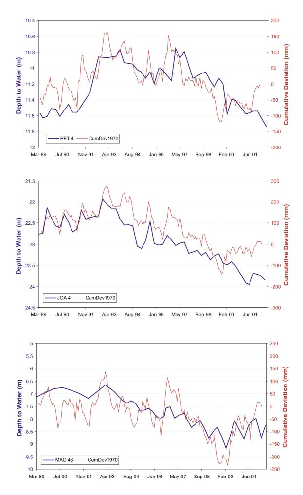
**Figure 12** Unconfined aquifer hydrographs compared to cumulative deviation (taken from data collected in 1970)
