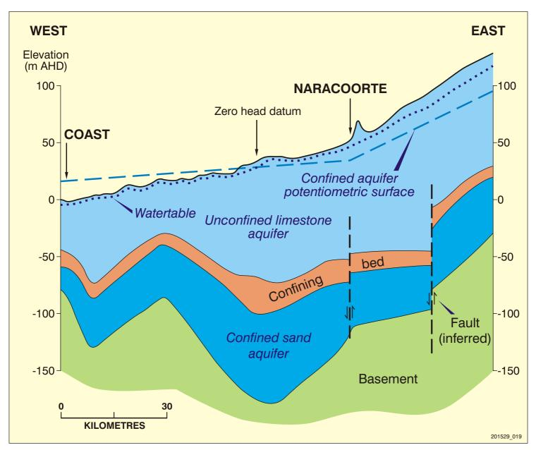
Figure 3 Schematic cross-section of southeast groundwater.
