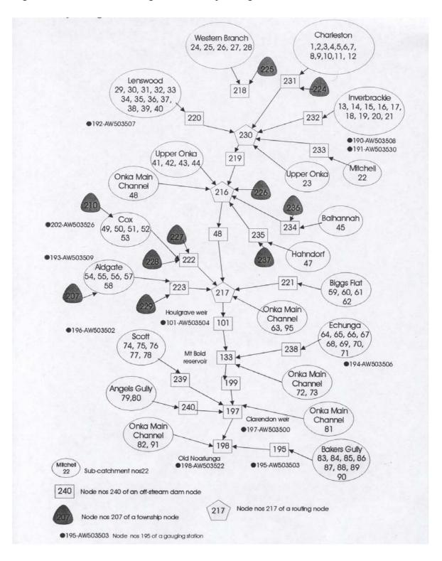
Figure 31. A Schematic Diagram of the Hydrological Model Catchment Nodes
