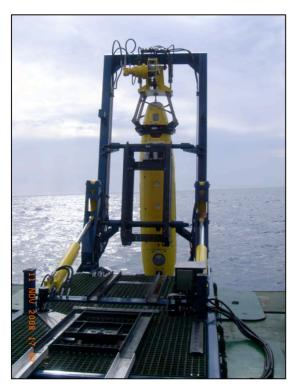
Fig.3: AUV ABYSS placed in its Launchand recovery system (LARS).
