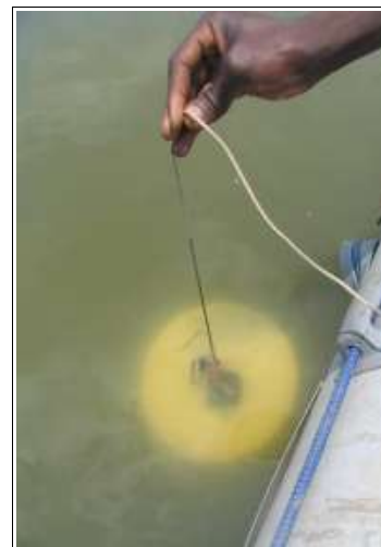
Figure 14: Measurement of water clarity with Secchi-disc (photo: Beate Böhme)
