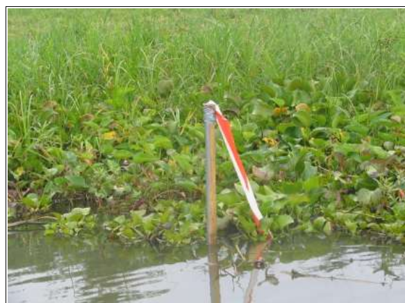
Figure 12: Lake level gauge at Lake Urema (photo: Beate Böhme)
