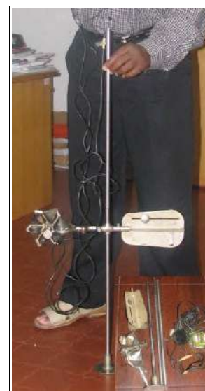
Figure 13: Current meter (photo: Beate Böhme)
