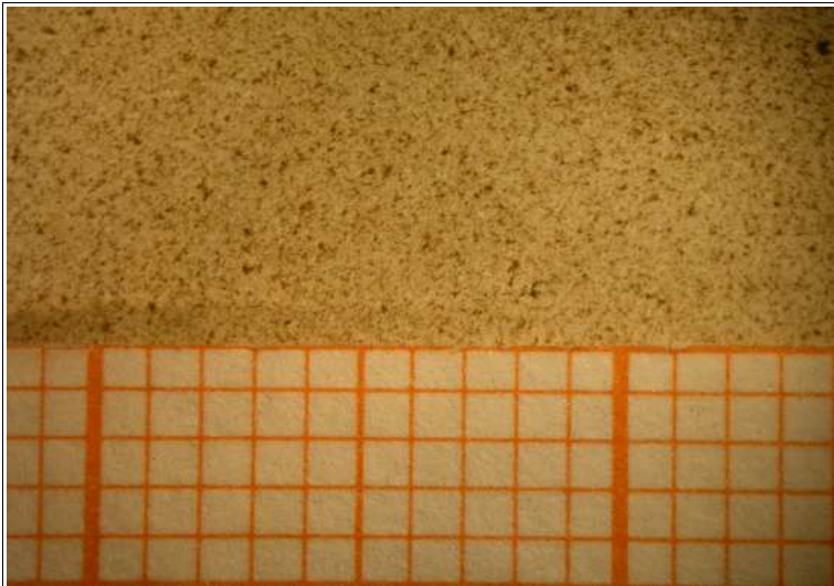
Figure 45: Top view at a water filter (200 nm mesh size, magnification 8 x) after filtration of 90 ml water from site 115, lower half of picture shows scale paper: box equals to 1 mm 2 (photo: Beate Böhme)
