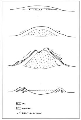
Figure 1: Scematic outline of growth and decay of a frost mound. The youngest part is at the top, and the age of the form increases downward of the figure.
