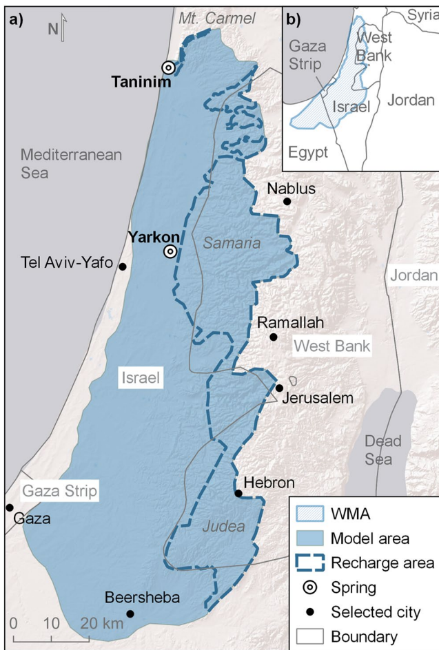
Figure 1. (a) Overview map of the model area located within the Western Mountain Aquifer (WMA) indicating the two major springs and recharge area of the karst system. (b) Regional overview and outline of the whole karst aquifer.
