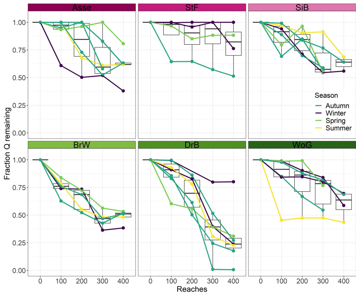
Figure 4. Fraction remaining of upstream discharge (site 0 m) at downstream sites along the 400 m reaches for all streams and seasons each (agricultural — upper panels, forested — lower panels). The slope of the curve depicts the magnitude of turnover along the reach, that is, it is high with a negative slope and is low to stagnant when the slope is positive or zero. The box plots depict the variability across all campaigns for each subreach along the study reach.
