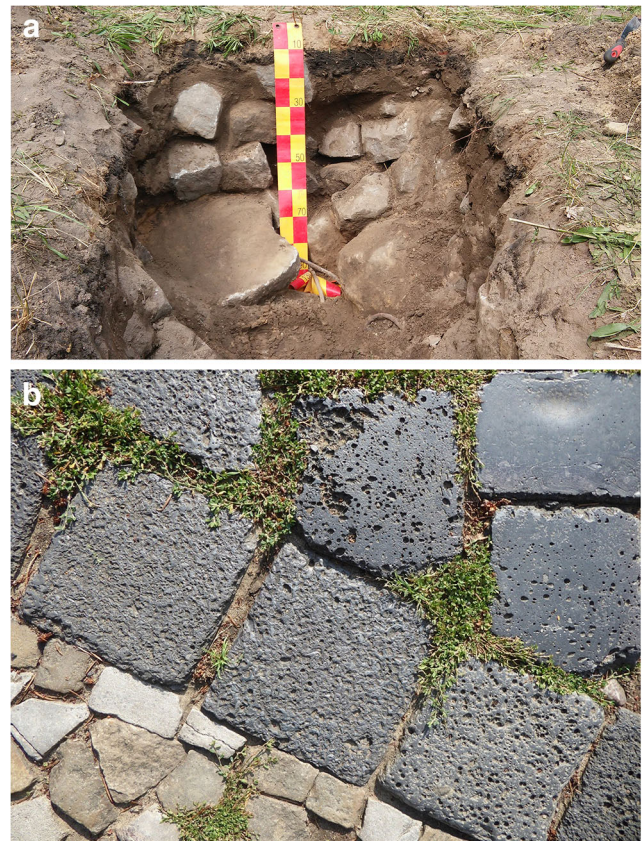
Fig. 5 (a) Soil profile on a former shooting range site consisting of different technogenic and anthropogenic materials, 0–10 cm, anthropogenic A horizon (natural soil material); 10–18 cm, technogenic C horizon (bitumen or tar); 18–60 cm, technogenic C horizon (construction sand + granitic pavement stones); > 60 cm technogenic C horizon (calcareous construction sand + ferro concrete). (b) Copper slag as paving stones, photos by K. Thestorf
