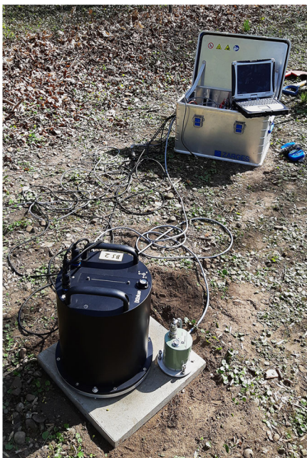
Fig. 2 Setup for the single station six-component noise measurements. The two instruments, the blueSeis-3A rotational sensor on the left and the Trillium Compact 120s seismometer on the right, are placed about 10 cm apart on a concrete slab. The instruments are connected to GPS, power, and the seismometer to a REFTEK digitizer (inside of metal box). Before starting the recording of the data, a styrofoam insulation box is placed over the instruments
