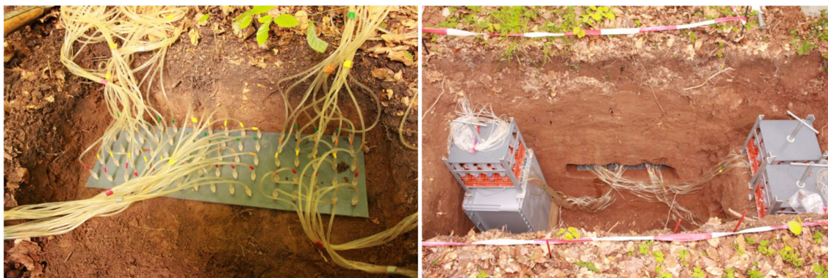
Fig. 1 Injection of DOC at 10 cm depth at the Red Sandstone site (left) and in 50 and 100 cm depth at the Loess site (right). Note that on the right site, the injection at 100 cm depth is
