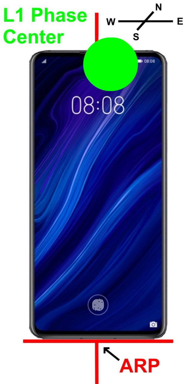
Fig. 6 Definition of the antenna reference point (ARP) and reference orientation; L1 phase center of Huawei P30 GNSS antenna
