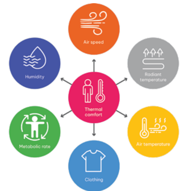
Figure 10.2. Parameters that determine the feeling of thermal comfort (Source: Design by Christina Karagianni, 2022)
