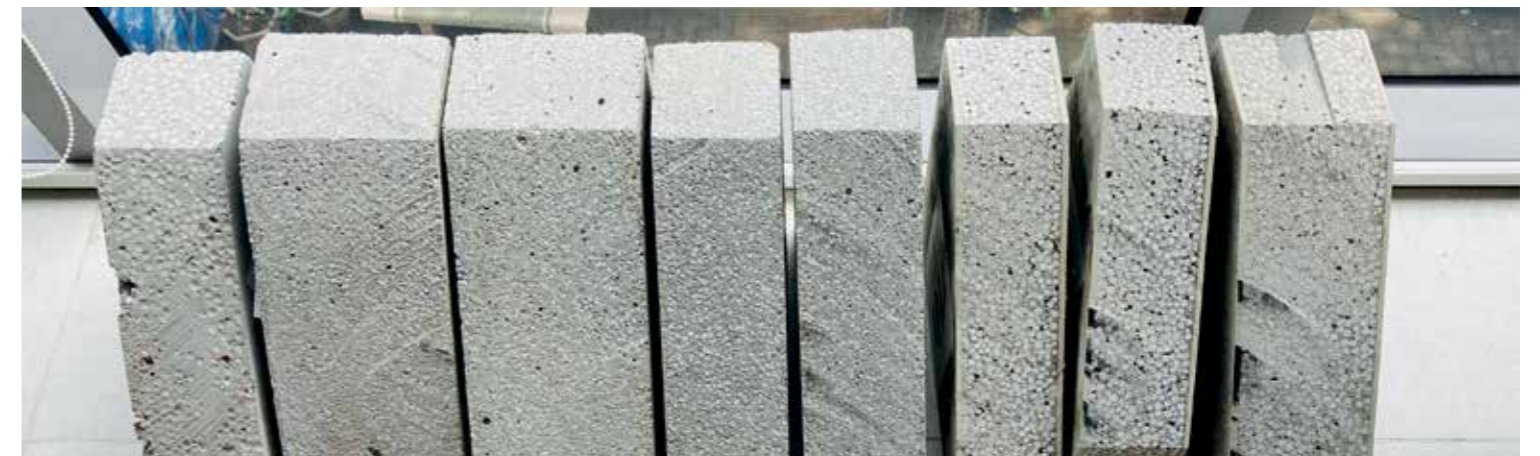
Figure 5.3. Development of Expanded Polystyrene (EPS)-based light-weight concrete sandwich wall panels "NUCEWALL" at Hanoi University of Civil Engineering (HUCE) (Source: Andreas Zegowitz)
