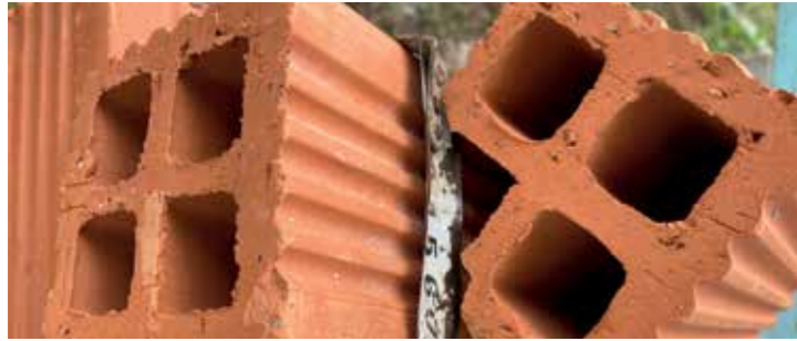
Figure 5.4. Air chambers in the building blocks increase the thermal insulation effect (Source: Andreas Zegowitz)
