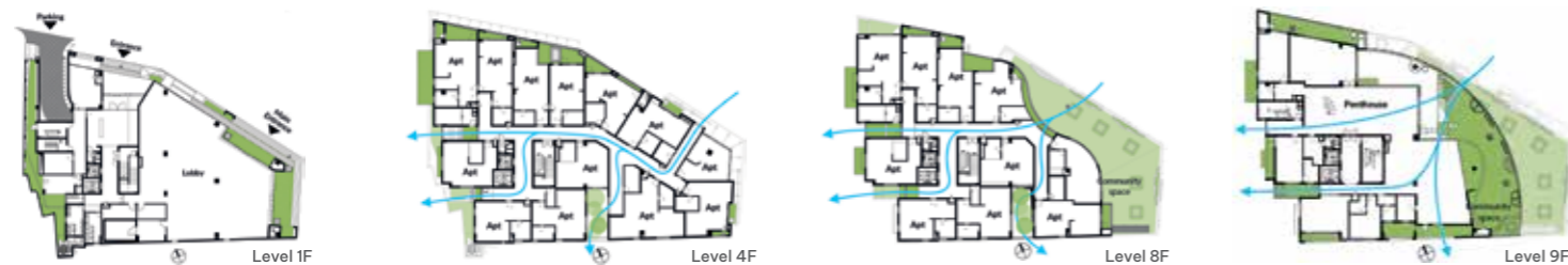
Figure 10.6. Building designed with natural ventilation (Source: 1+1>2 Architects)
