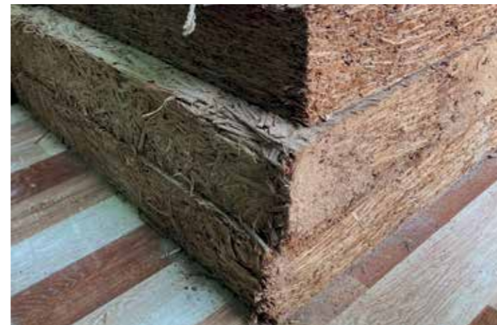
Figure 4.2. Example of bio-based building material: Coconut fiber (Source: Michael Waibel)
