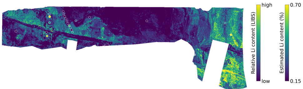
FIGURE 10 Predicted Li grade for outcrop Z1 derived by multiplying the zinnwaldite abundance by its average Li content (1.7%). White outlined circles show relative (uncalibrated) Li values from the independent LIBS measurements. For the 3D version of this map, see https://tinyurl.com/Zinnwald .
