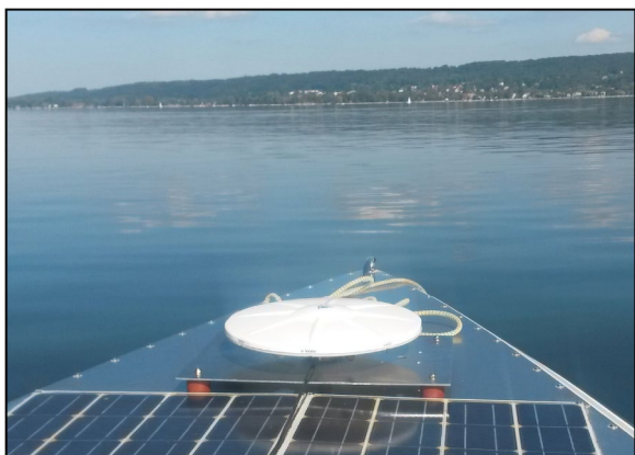
Fig. 10 Picture of the Trimble Zephyr 3 Geodetic antenna used for recording the observation during the test at the Lake Ammer (southern Bavaria)
