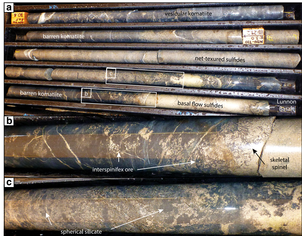
Fig. 4 a Drill hole MDU-710 from the central parts of McLeay showing a typical profile of Lunnon Basalt followed by massive sulfides, komatiite with minor irregular sulfide patches, net-textured sulfides and barren komatiite. b Close-up of (a) to show the contact of massive sulfides to komatiite which hosts the interspinifex ore. c Close-up of (a) to show the upper contact of the komatiite with patchy sulfides to the net-textured sulfides above.
