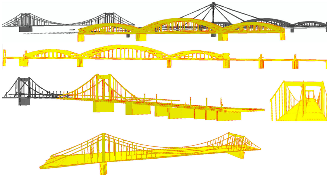
Fig. 26 Large bridges in Cologne: superstructures were reconstructed using the Hough transform combined with histogram-based column completion on projection images. Yellow bridges from top to bottom and left to right: Hohenzollern Bridge, South Bridge, Mülheim Bridge (based on two cadastral footprints), two images of Rodenkirchen
