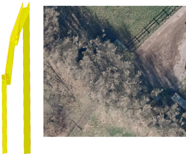
Fig. 20 The bridge is completely covered by trees. As a result, the z-coordinates of the deck are wrong
