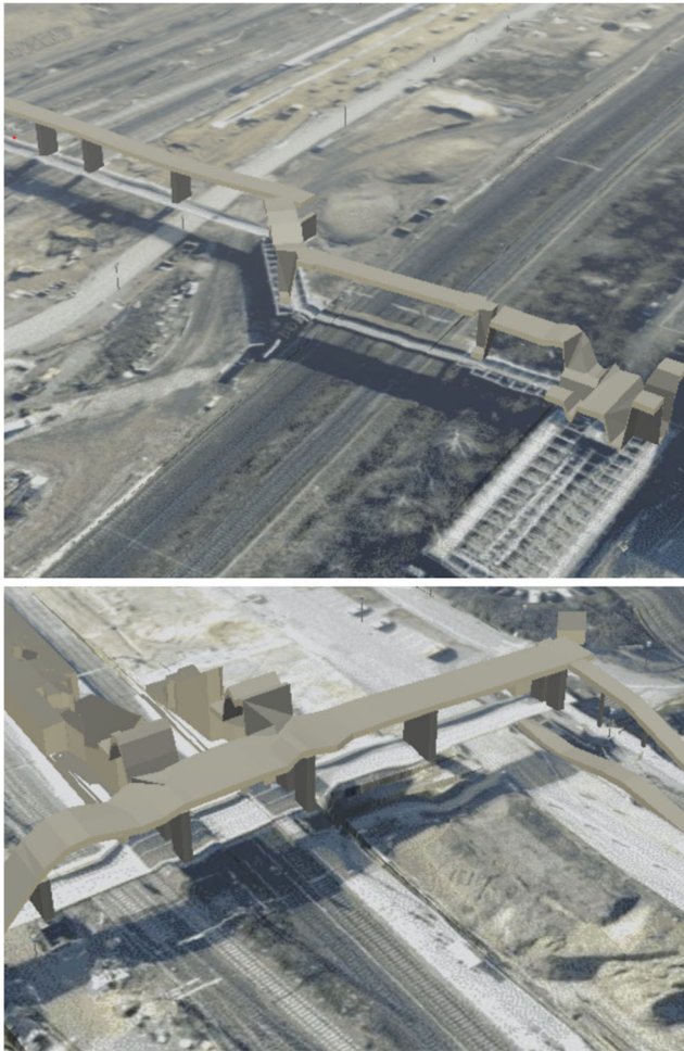
Fig. 24 Roofs lead to wrong z-coordinates of decks of pedestrian bridges at a railroad station
