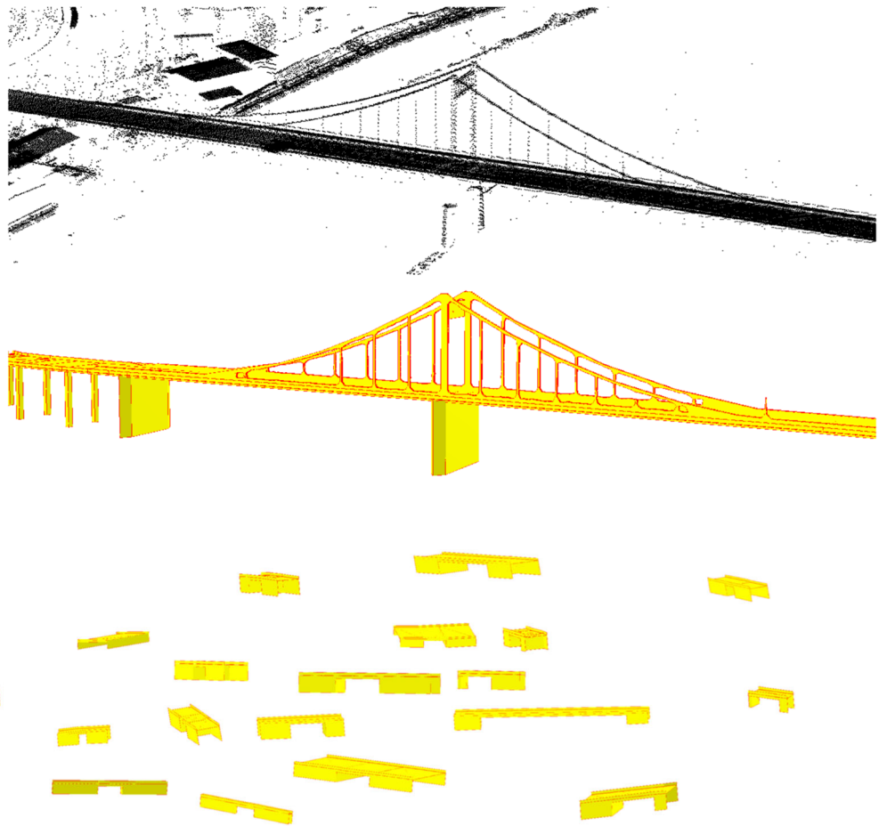
Fig. 14 Most bridges have a simple structure. In the examples, counter bearings are extended to fill gaps between floating parts and ground
