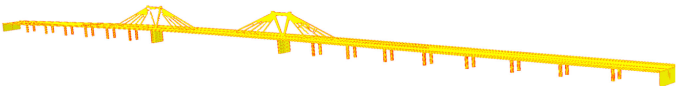
Fig. 10 Motorway bridge (Düsseldorf Airport Bridge) with a superstructure along the medial axis and multiple pillars from cadastral data
