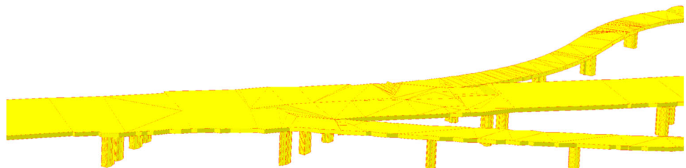
Fig. 2 Up and down ramps lead to branches: The bridge was reconstructed based on a tree obtained from a medial axis
