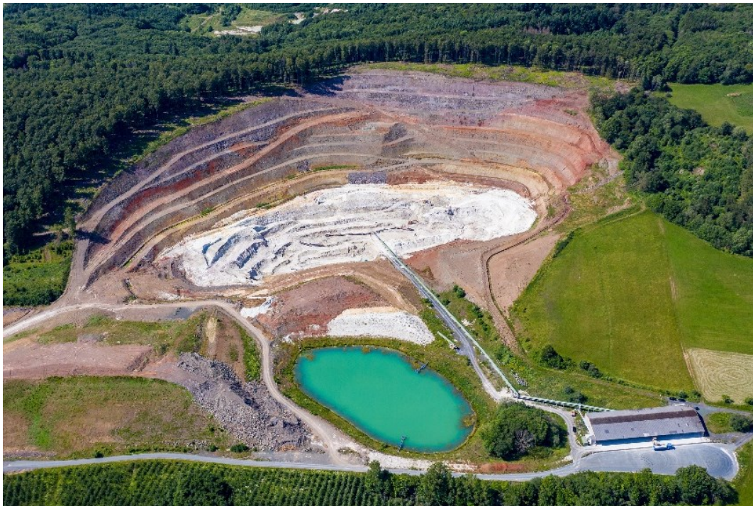
Figure 1. Mine Wimpsfeld 3, white kaolinitic-illitic clays with an overburden of bentonites and basalt. – Picture: Stephan Schmidt Group
