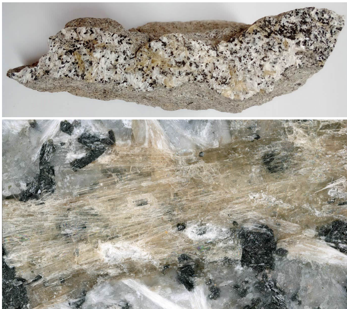
Figure 1. Yellowish brown crystals of götzenite and wöhlerite in association with natrolite (white) and clinopyroxene (black). Widths of figures are 11 cm (top) and 5.7 mm (bottom), respectively.
