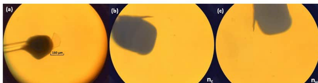
Figure 1: (a) \text{KBrO}_3 crystal mounted on the spindle stage of the polarization microscope. (b) orientation of the crystal to determine n_e = 1.538 . (c) orientation of the crystal to determine n_o = 1.677 . Due to the equality of the refractive indices of the sample and the immersion oil, the sample is not visible in (b) and (c).
