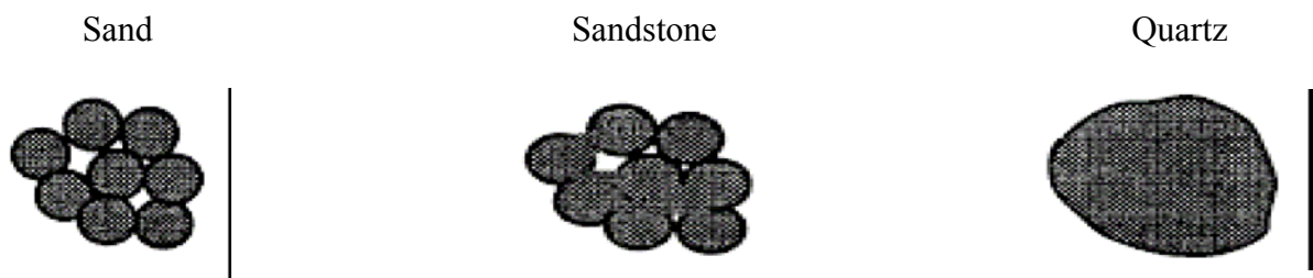
Figure 2: Schematic diagrams showing the evolution of the porous structure during the diagenesis of quartz. As diagenesis progresses, sand grains become compacted and cemented. The initial porosity (40 %) decreases down to zero. Modified after Nur et al. [63].
