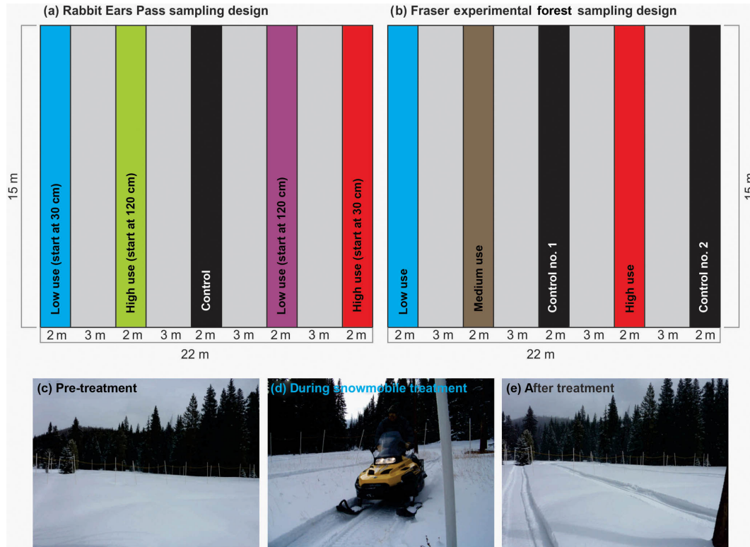
Figure 2. The sampling design for the snow compaction plots at (a) Rabbit Ears Pass, (b) Fraser Experimental Forest, and photographs of the study plots (c) pre-treatment, (d) during treatment, and (e) after treatment. The colors used for the control and treatment plots are used in Figs. 5–8.
