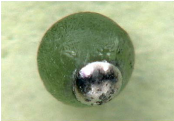
Figure 14 Photography of the reduced lherzolite-metal oxide mixture. Metal exsolved from the silicate. The diameter of the sphere was ~2 mm. The material was levitated with a mixture of 98 vol.% Ar and 2 vol.% H 2 .
