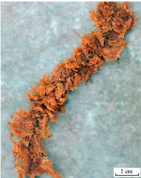
Abb. 7: Subrezentes Moos aus Sphagna cymbifolia -Torf, Humifizierungsgrad 2 Subrecent moss from Sphagna cymbifolia peat, degree of humification 2
