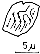
Fig. 9: Sketch of the domain structure of a four domain particle in the Rauher Kulm basalt with bent domain walls. Dot: etch pit due to a dislocation intersecting the surface.
