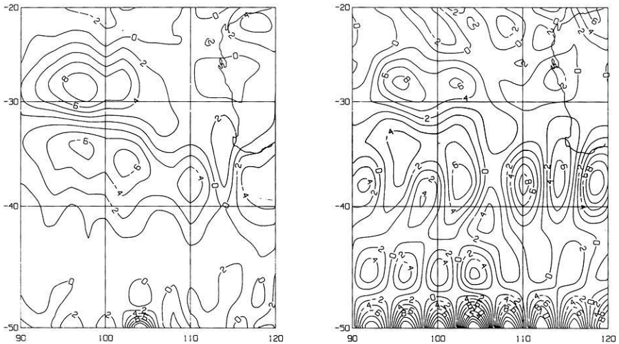
Fig. 7. 1^\circ average anomaly data (left) and magnetization distribution (right) from inversion of this data. Units are nT (left) and 10^{-1} \text{ Am}^{-1} (right)
