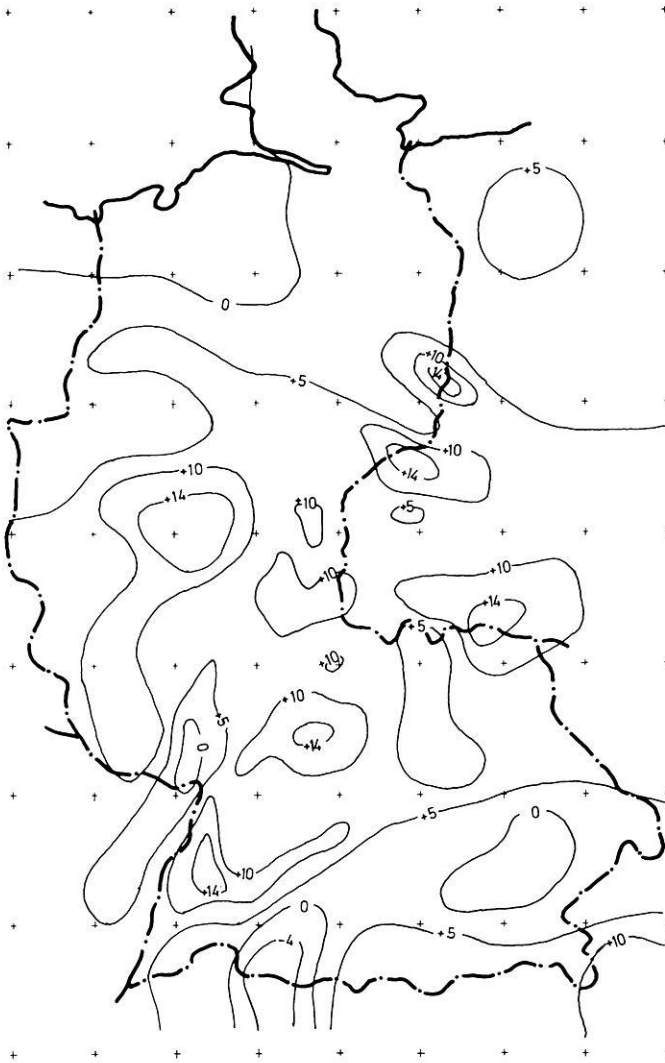
Fig. 6. Lateral density variations ( 10^{-3} \text{ gr cm}^{-3} ) in a lithospheric layer of thickness H = 100 \text{ km} corresponding to free air anomalies of flattening 1/298.25 in F.R. Germany
