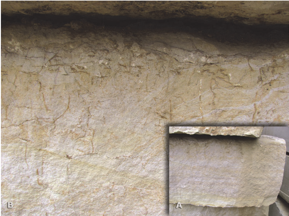
Fig. 6 One of the typical root-trace horizons from the Obernkirchen sandstones (A), showing the strictly vertical orientation without any horizontal layering or subdivision (B).
